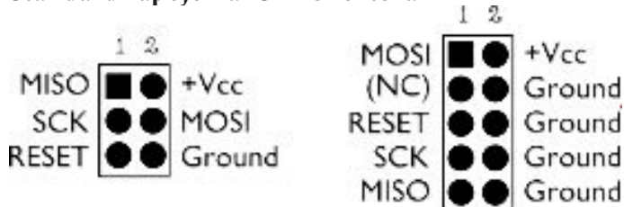
ISP Connectors: 6-pin & 10-pin
